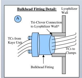
\*Note: Bulkhead is capable of interfacing with the Lyophilizer wall through various connection types (e.g. Tri-Clover, Threaded, etc.)
